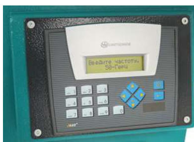
SM 2.0 shaker mixer control panel
