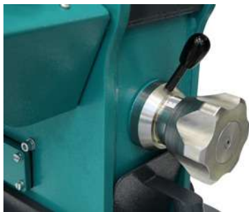
Device for adjusting gap between jaws of JC 6M
