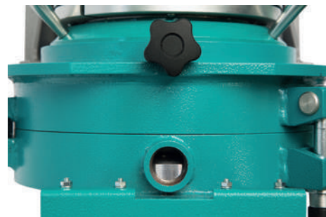
Opening for monitoring gap between discs
