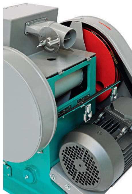
Pipe for connecting dust collector and cleaning window
