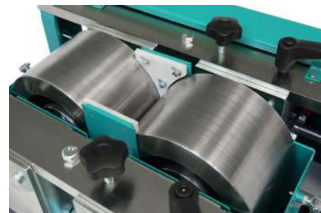
Rollers and fluoroplastic liners
