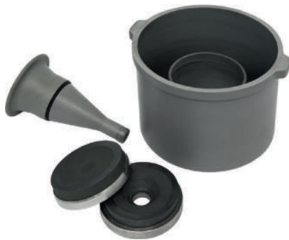
DG 65 charging funnel, receiving container and discs
