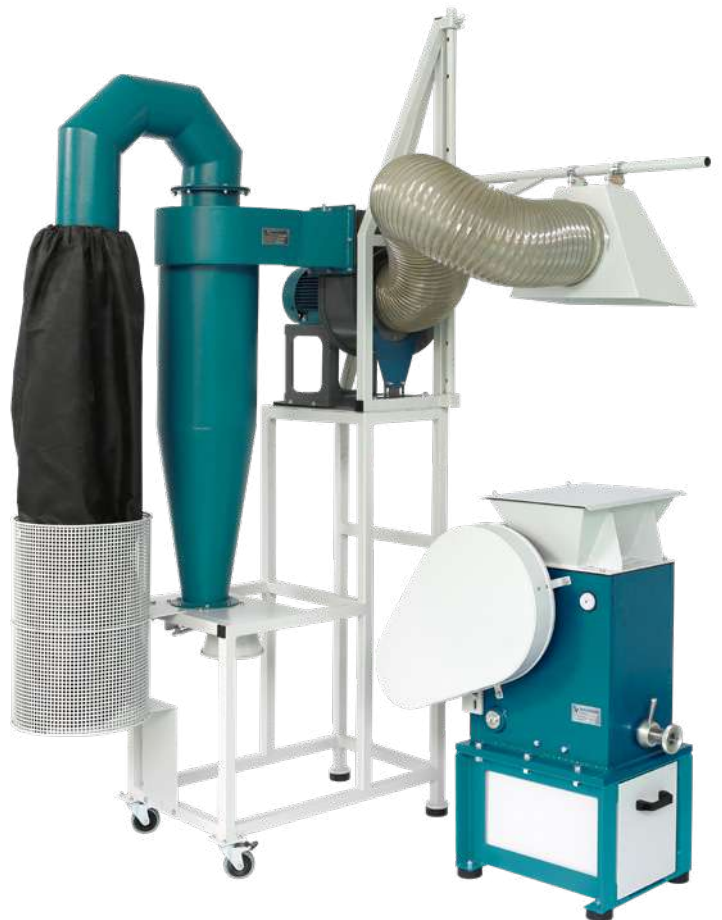
Cyclone dust collector with hood and Jaw crusher JC 10
