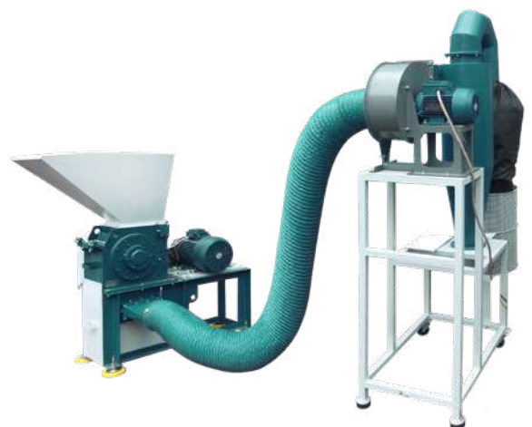
Cutting mill CM 250 with Cyclone dust collector
